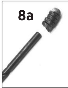
Photos 8 and 8A Take the double flattened end piece and wrap it around a 3/16 rod of some sort to make a coil. I used the end of a drill bit holding it secure with a cloth so it would not slip and injure my hand.
